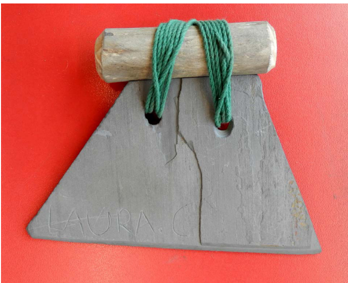
Figure 6: An example of a how string should be tied around the handle to secure the slate blade.
