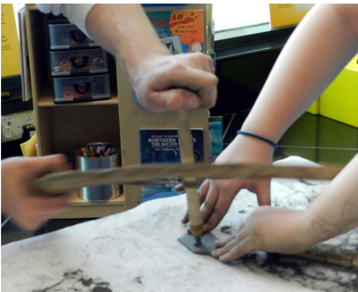
Figure 5: The spindle should spin straight up and down and downward pressure is applied through the hand holding the socket piece.
